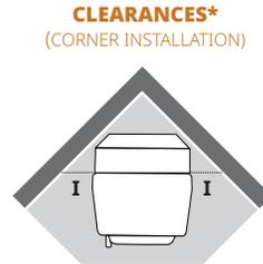
\*When using 3" PL vent pipe, there must be 3" clearance to combustibles.
