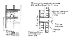
Minimum chimney clearance from masonry to sheet steel supports and combustibles 2 in, (51 mm)
