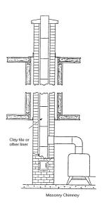
Be sure that all connectors between the chimney parts and the heater are sealed properly so the chimney is airtight from the heater to the chimney outlet.
